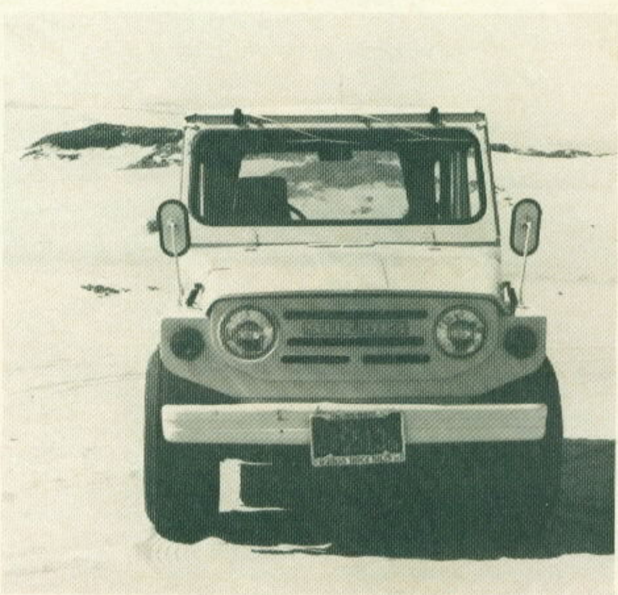
Overall height is 64.8 inches at the windshield and length is 117.9 inches. Total weight for the Suzuki Brute IV, unloaded, is 1350 pounds.
